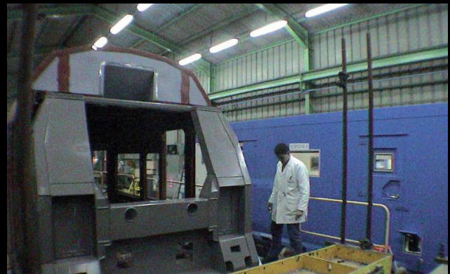
Experimental analysis on a complete bodysell (up to 100 channels)
