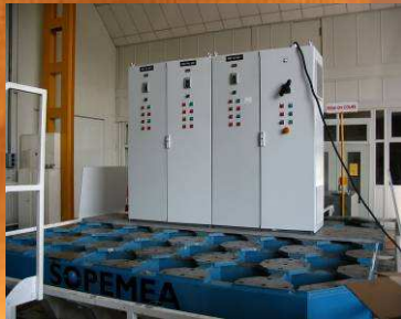
Electrical bay seism simulation
