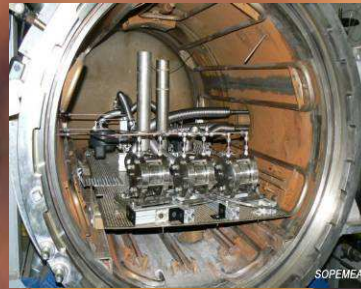
Thermodynamic accident on pressure pick-ups
