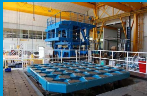
Hall dédié aux essais de vibrations Hall dedicated to electrohydraulic vibrations test
